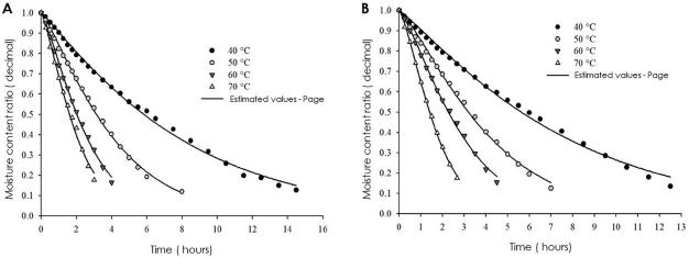
**Figure 2.** Moisture content ratios of pumpkin (*C. moschata* Duchesne) seeds of the genotype 'AC 53' (A) and the cv. 'Goianinha' (B), obtained experimentally and estimated by Page model, for various drying conditions.
