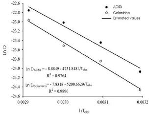
**Figure 4.** Arrhenius representation for the effective diffusion coefficient as a function of drying air temperature, obtained during drying of pumpkin (*C. moschata* Duchesne) seeds of the genotype 'AC 53' and the cv. 'Goianinha'.
