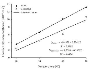
**Figure 3.** Effective diffusion coefficient obtained for the drying of pumpkin (*Cucurbita moschata* Duchesne) seeds of the genotype 'AC 53' and the cv. 'Goianinha'.
