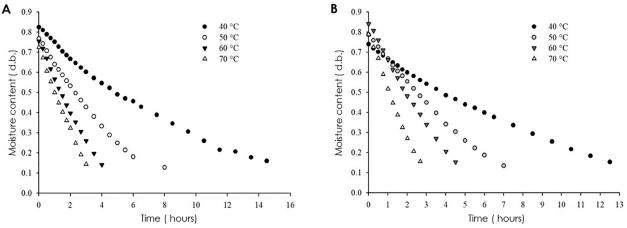
Figure 1. Drying curves of pumpkin seeds genotype 'AC 53' (A) and cv. 'Goianinha' (B) at temperatures 40, 50, 60 and 70 °C.
