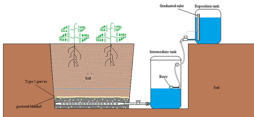
**Figure 1.** Illustration of the groundwater lysimeter built inside the protected environment.
